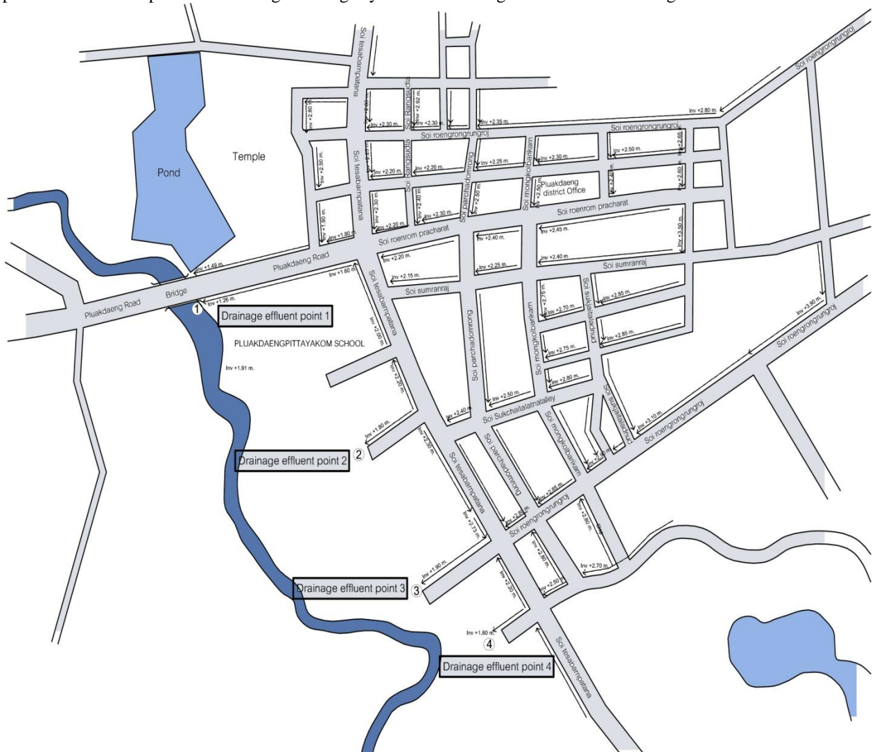
Figure 2. Drainage systems in Pluakdaeng municipality.
